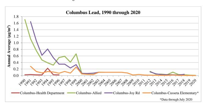
As of 2018, GA AAMP operated two lead monitors in the Columbus, GA-AL MSA. The next graph is a comparison of the 2018 through 2020 monthly averages, showing the difference between when the emission source was in operation (solid lines) to when it was shut down (dotted lines).
