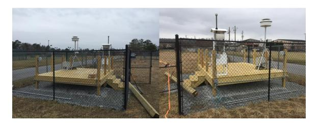
Preliminary measurements were made at the site to ensure that the sampler is at least 10 meters from any trees and that the sampler has 270° unobstructed fetch for wind flow, and indicate that the sampler meets the siting criteria in 40 CFR 58, Appendix E. The information below shows the site details for the new Columbus-Baker monitoring station.
