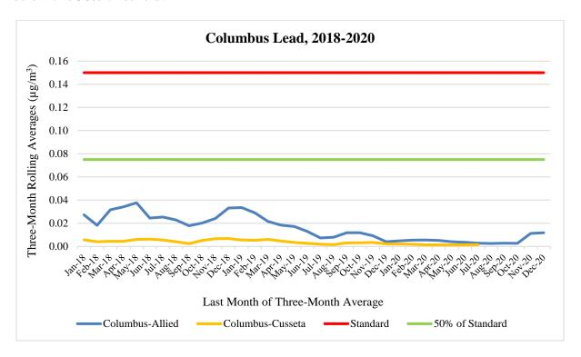
With the source no longer producing lead, and the lead data well below 50% of the standard, the GA AAMP is requesting to discontinue monitoring for lead in the Columbus, GA-AL MSA as of December 31, 2020. The GA AAMP will keep the lead monitors in place for a time in case a need arises to monitor lead in the Columbus, GA-AL MSA in the future.
